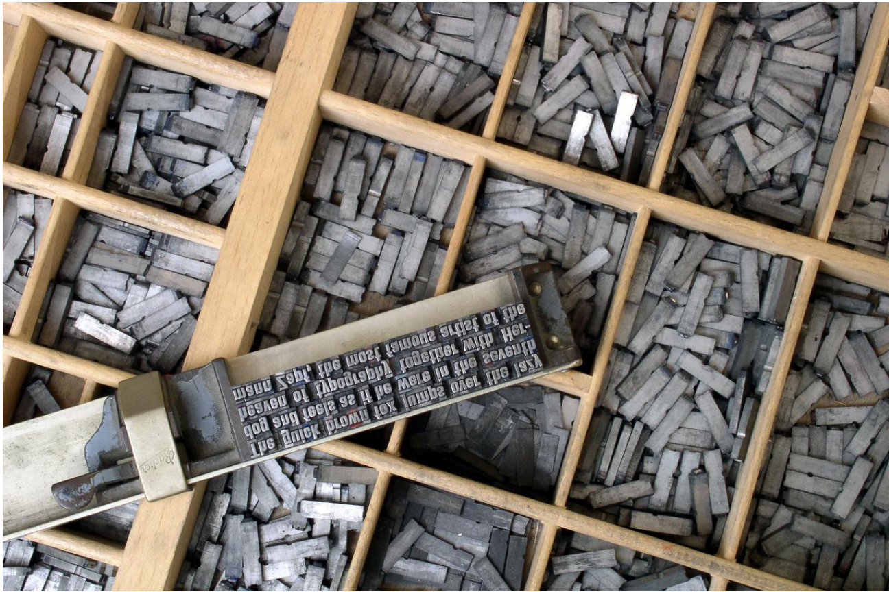
Movable type sorted in a letter case and loaded in a composing stick on top.
